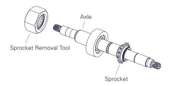
2 Using the pliers on the sprocket, unscrew the sprocket from the axle.
