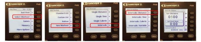
• After completion, view the memory and note the average pace. This will be the average pace of a single distance OR the combined average pace of all the work portions of an interval workout.
